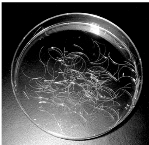
FIGURE 2 Photograph of self-supporting assembly of silica particles on petri dish (diameter of silica particles: 0.1\text{ }\mu\text{m} ).
